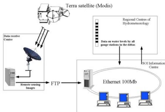
Figure 2. Scheme of communications during the “Vernal Waters” experiment.
